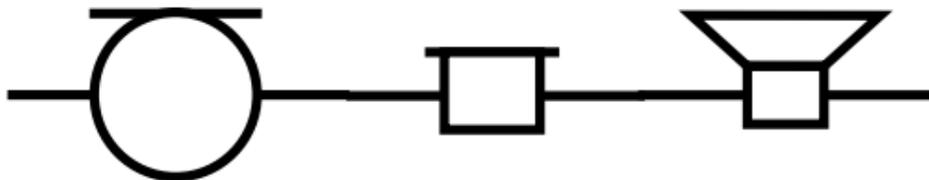
Microphone: 1-2. Common. 3. Condenser. 4. Piezoelectric.
